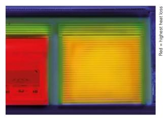
This thermal image of an ordinary roll-up door clearly shows the large heat loss to the outside.
