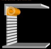
The round spiral is standard and the ideal solution when you have sufficient space above the door.
